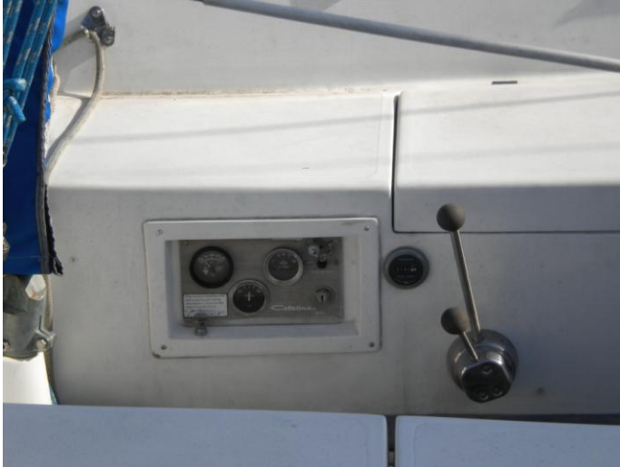
Engine Controls and Displays- large lever is engine gear
